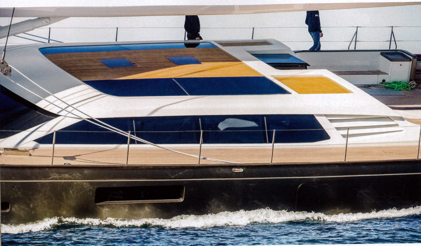
Let there be light: the deckhouse roof features both windows and skylights. The rectangular hull port shown is in the dining saloon.
