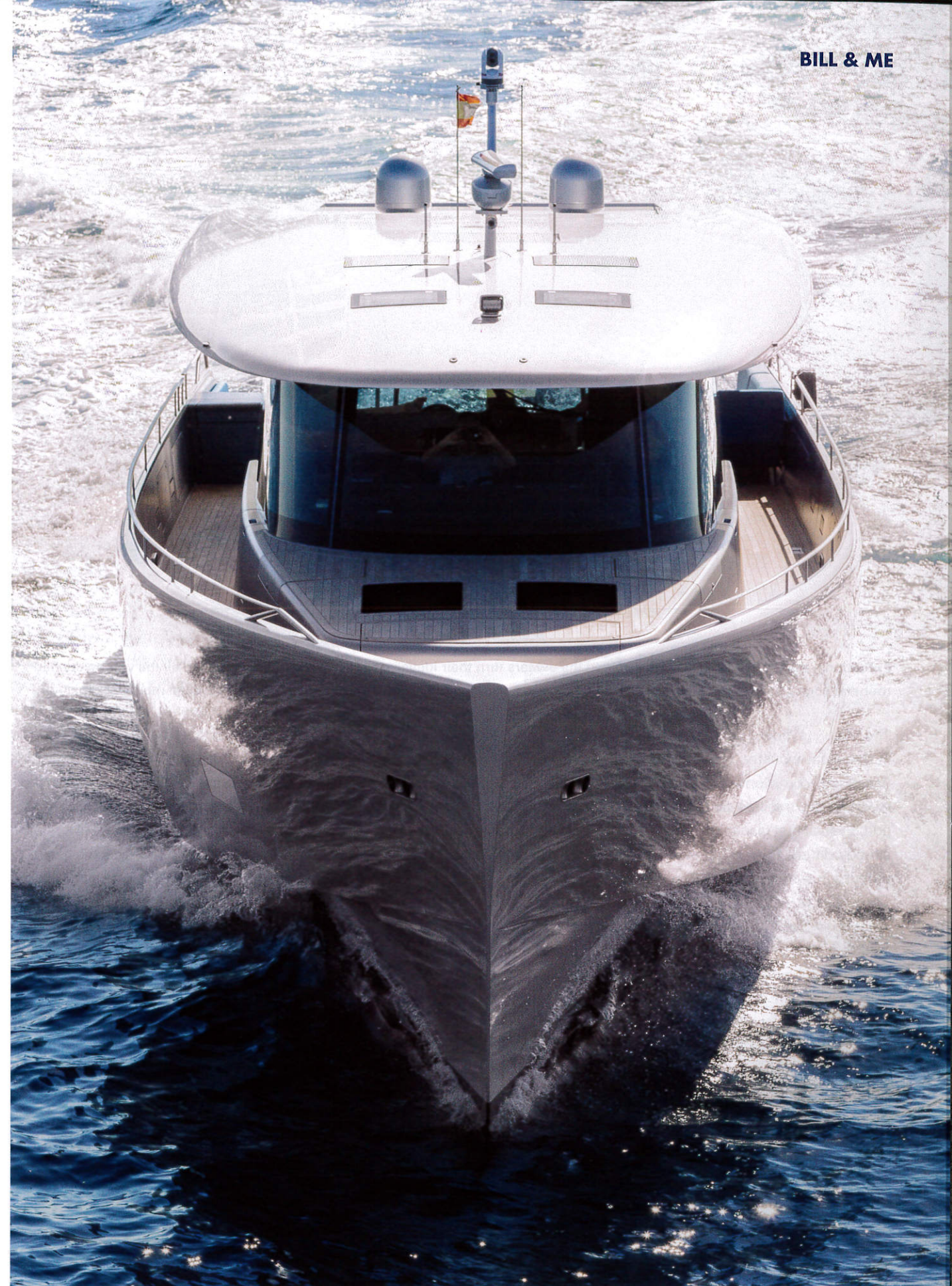
Speed: 40-tonne "Bill and Me" can cruise at up to 25 knots thanks to her IPS pod drives with twin counter-rotating propellers.
