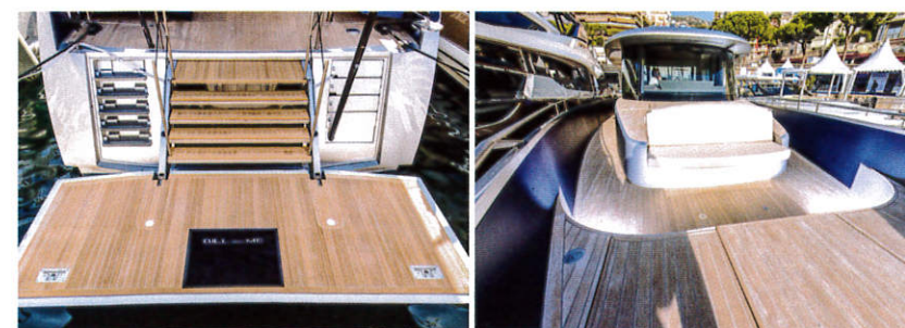
Flexible designs: the hydraulically operated transom can quickly be transformed into a swimming platform (left). The superstructure's forward edge folds into a sofa (right).
